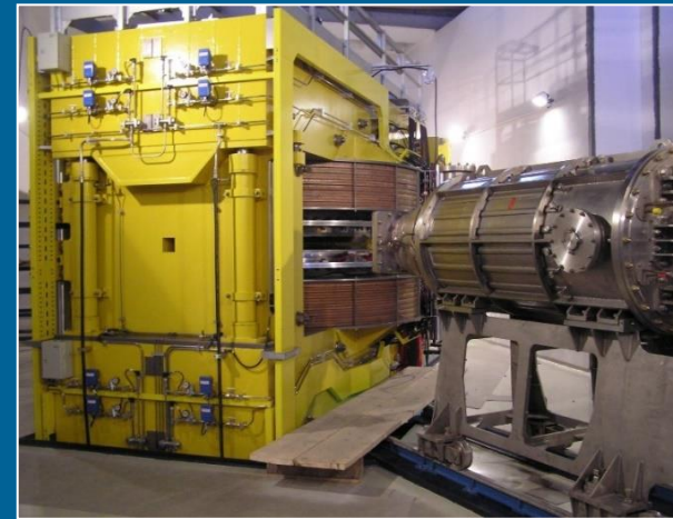
Main cyclotron of the TESLA Acceleration Installation complex aiming to deliver 70 MeV protons for the proton therapy, experimental production of radiopharmaceuticals and the analysis of materials.
