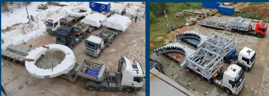
The yoke of the magnet consisting of 28 bars, supporting end rings and two pole tips weighs about 700 tons. 39 trucks transported all the elements of the yoke and beds from Czech Republic to JINR.
