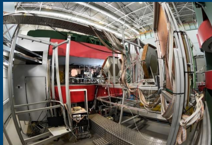
The yoke of the magnet consisting of 28 bars, supporting end rings and two pole tips weighs about 700 tons. 39 trucks transported all the elements of the yoke and beds from Czech Republic to JINR.
